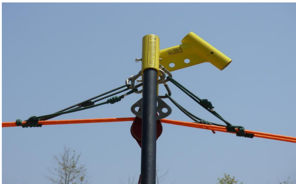
Figure 16-10. "A" frame centering prusiks (shown on AZV).
