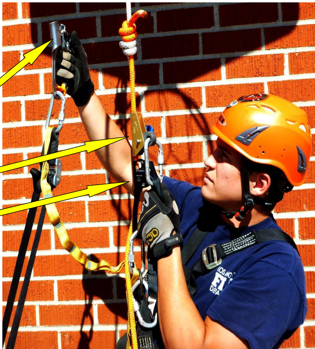
Figure 12-10. Removing lead ascender
