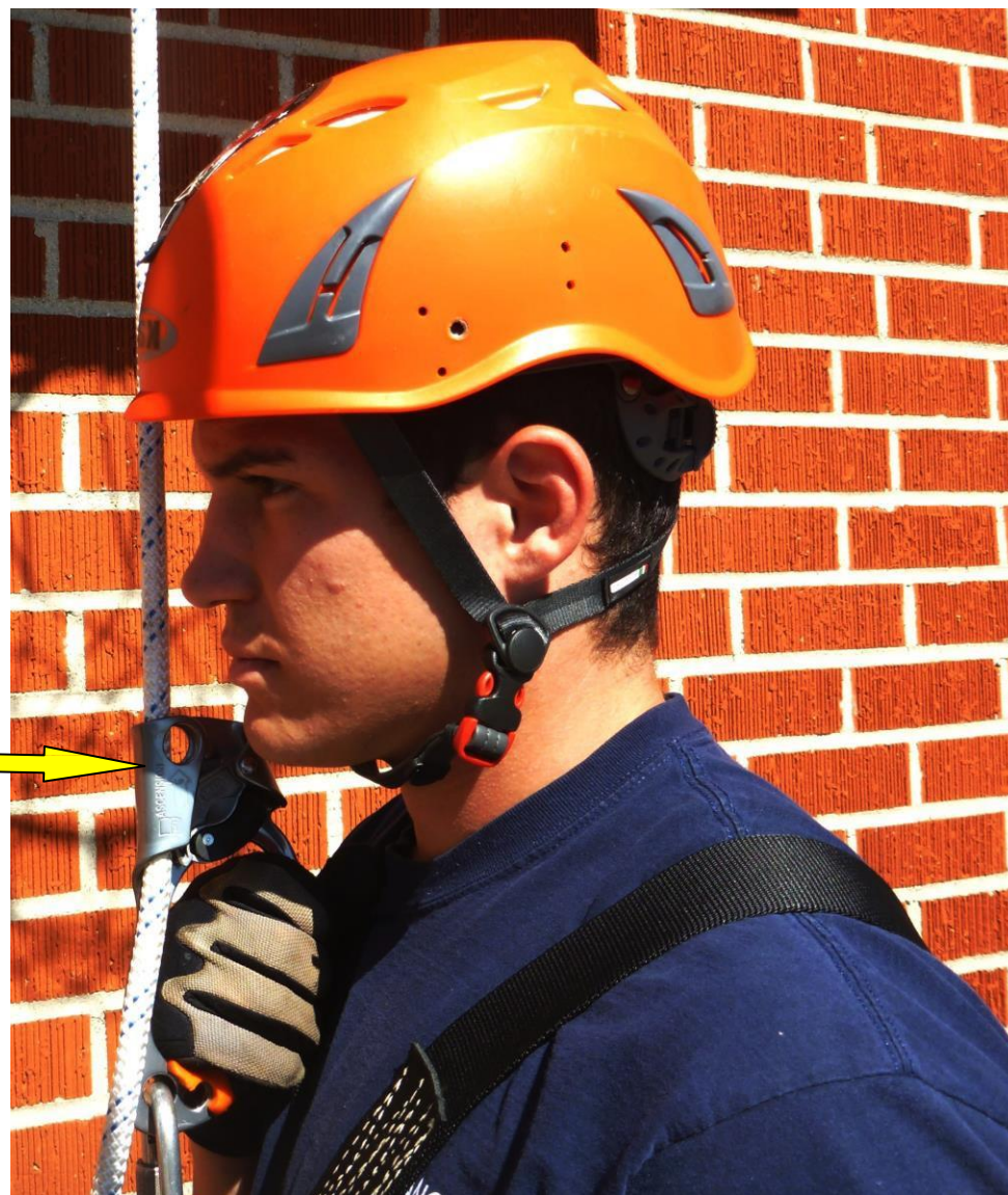
Figure 12-6. Adjusting Lead ascender
