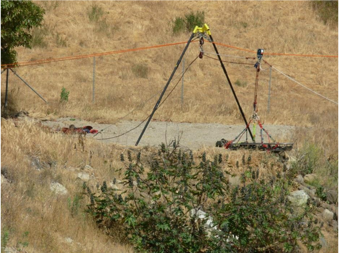
Figure 16-1. Artificial High Directional.
