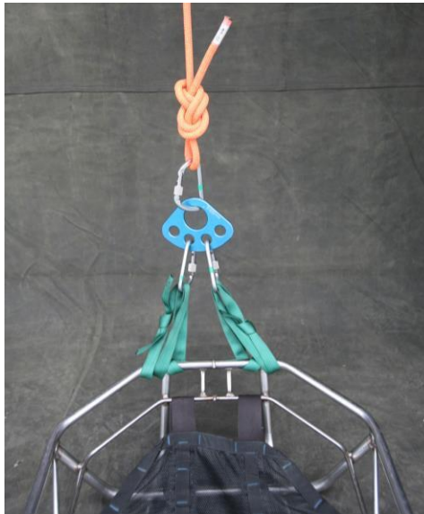
Figure 15-2. Litter rigged for a vertical lower/raise. Second line omitted for picture clarity.
