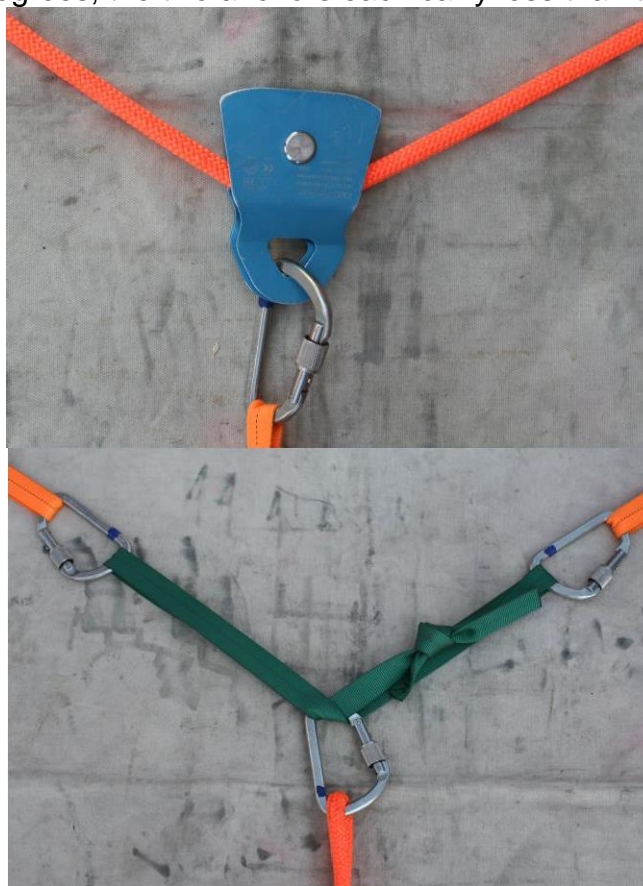
Figure 4-1. Two examples of 120 Degree Critical Angle
