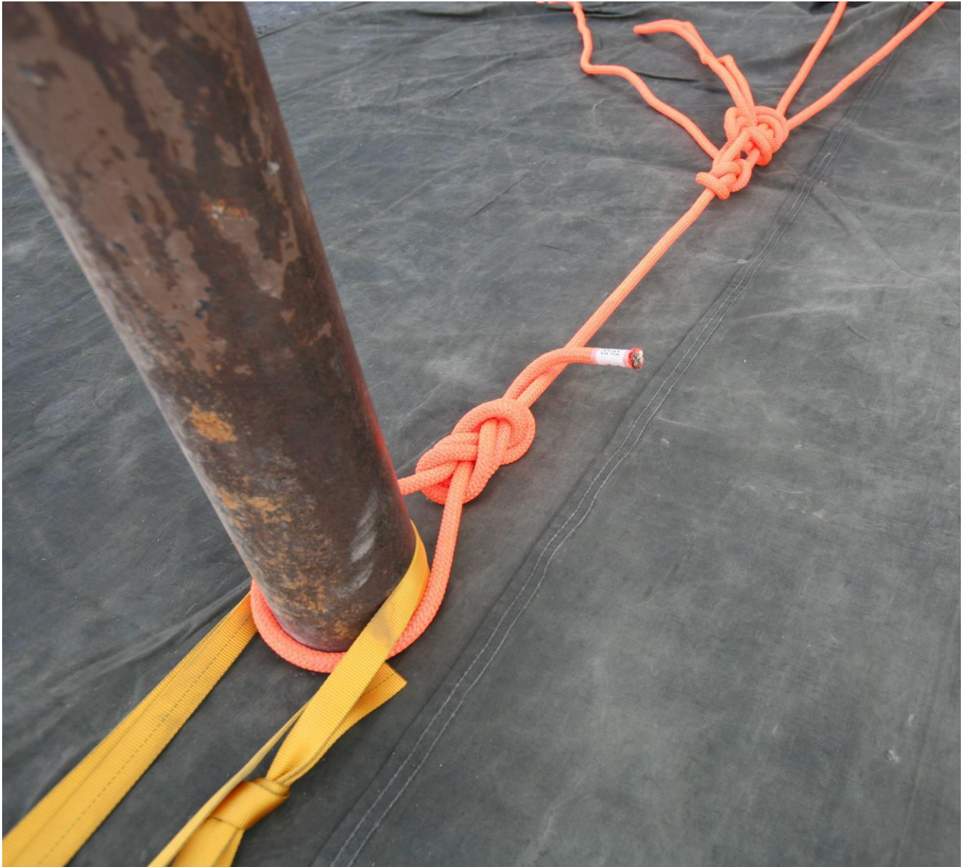
Figure 4-3. Back tied anchor.
