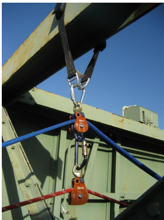
Figure 17-2. A Structural High Directional
