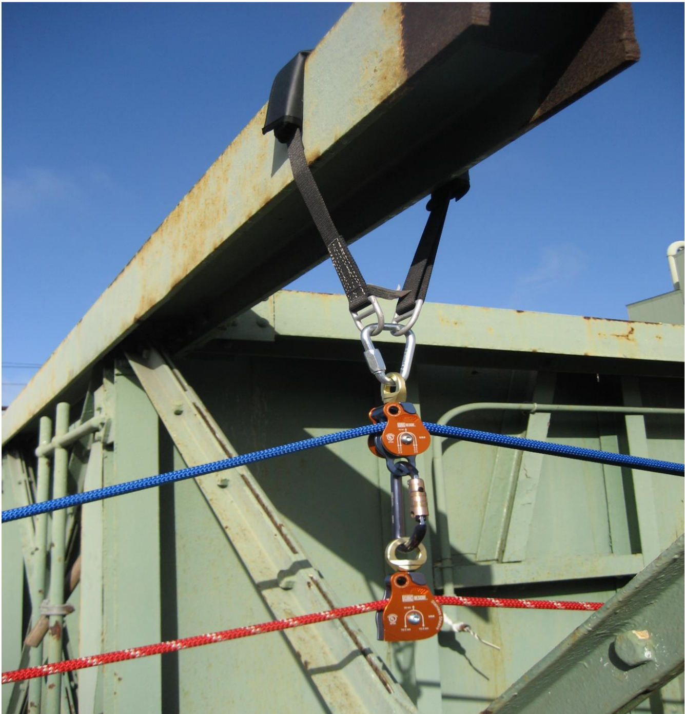
Figure 16-2. Structural High Directional.
