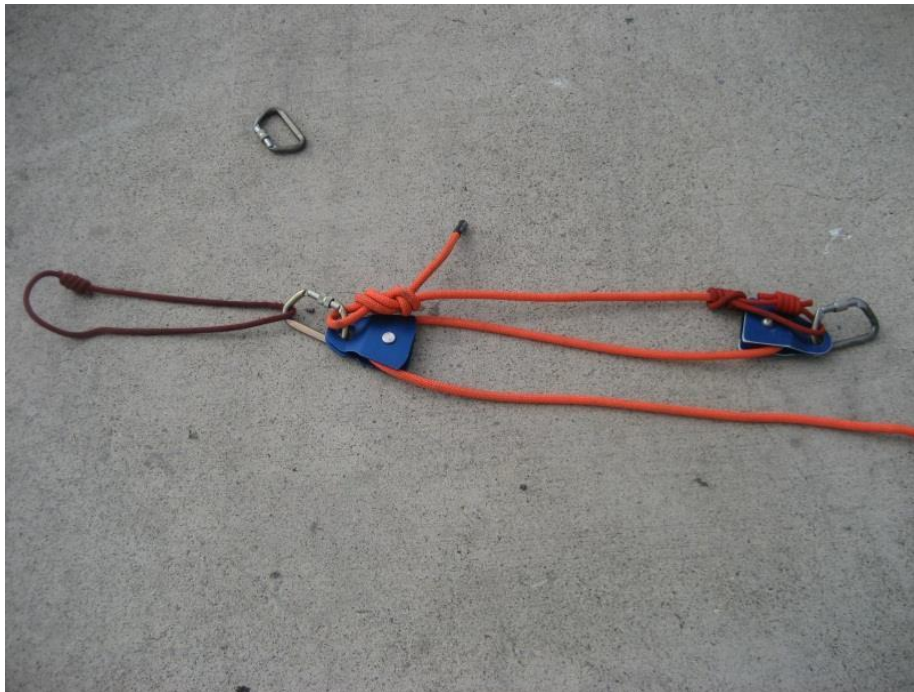
Figure 11-8. Pre-constructed 3:1 Piggy back.
