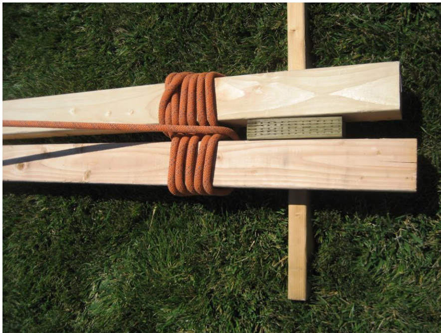
Figure 16-6. Wrapping and frapping.
