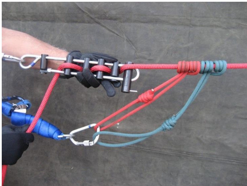
Figure 17-6. Tagline with Brake Rack and Tandem Prusiks
