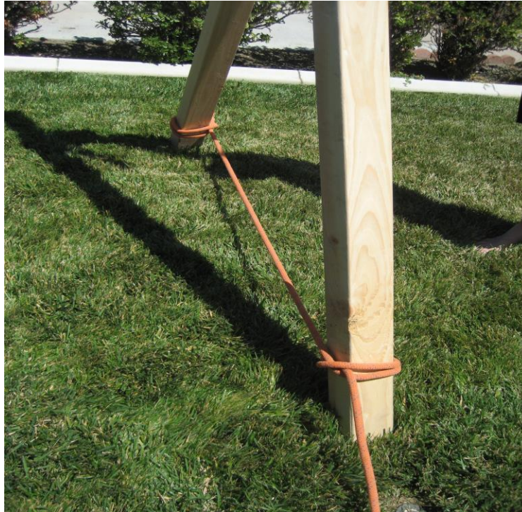
Figure 16-9. Hobble on legs of “A” frame.
